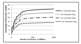
Figure 4.2.2: Results of Minimum Password Length and Requiring Digits on Longer Password Cracking Sessions
